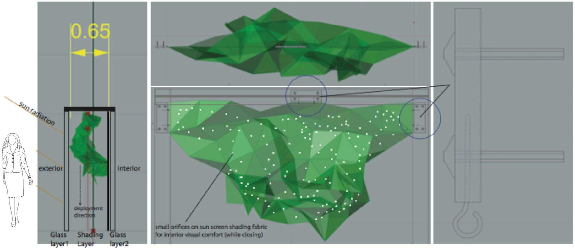
Details of Bio-inspired design shading device
