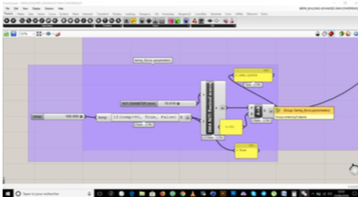
**SMM NiTi Flexinol Mecca:** a custom subroutine written in Grasshopper's Python editor, uses the  $(2ax^2))^c = F(x)$  pull force formula and combines it with Grasshopper's Unit Vector components to turn the values into proper vector form to enable the physical simulations
