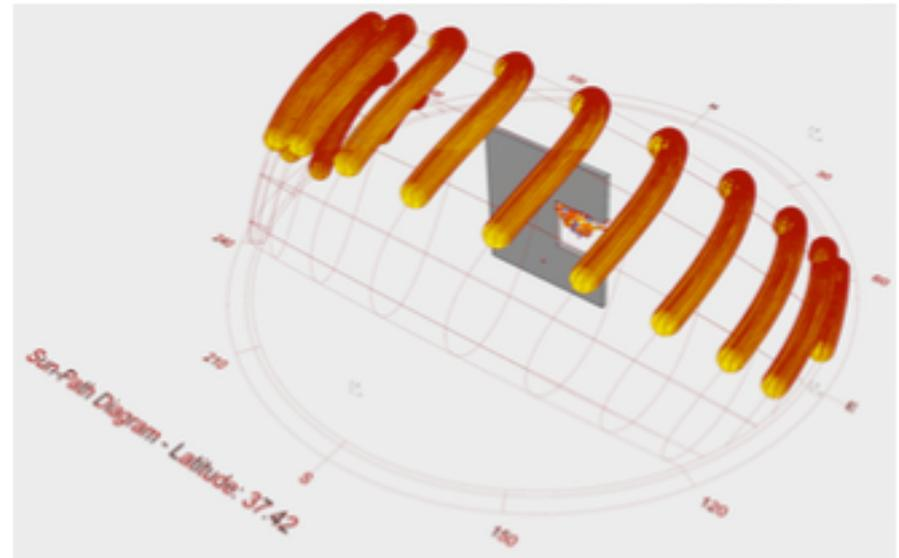
(left) Sun radiation analysis interacts with shading device area from 4::00h to 24:00h on August 1<sup>st</sup>
