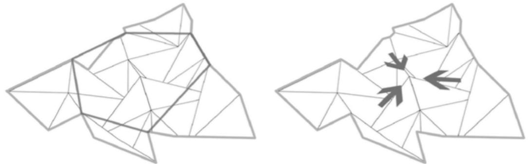
***The embedded SMA wires define the direction of deployment***
