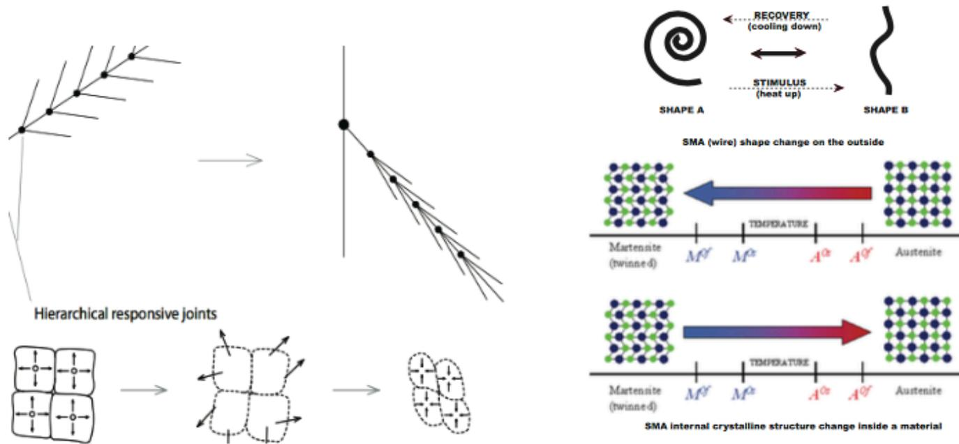
The comparison of mechanical change at macro scale and physical property change at micro scale between Mimosa Pudica leaves and the Shape memory alloy wire.
